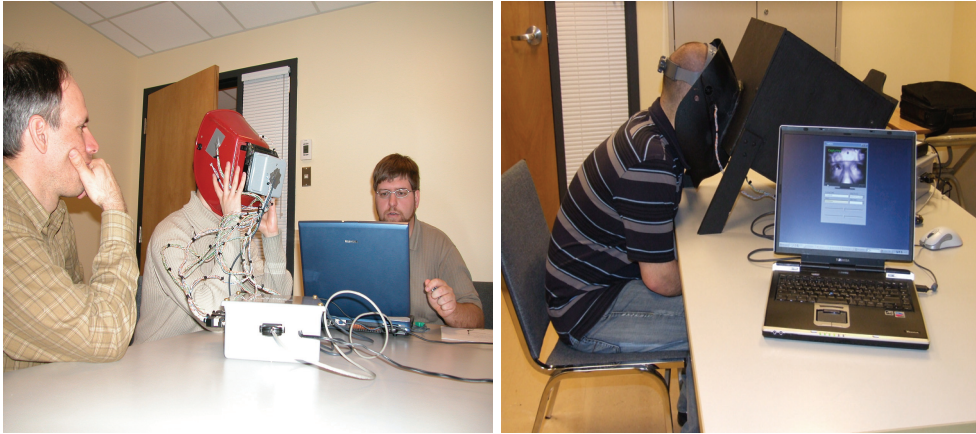
Fig. 8. Last two versions of the prototype. (Left) Previous version with automatic generation of visual stimuli. (Right) New version with enhanced visual stimuli generation and NIR illumination.
