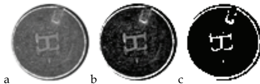
Fig. 13. Low-contrast image, a. Result of contrast enhancement, b. Result of threshold, c.
